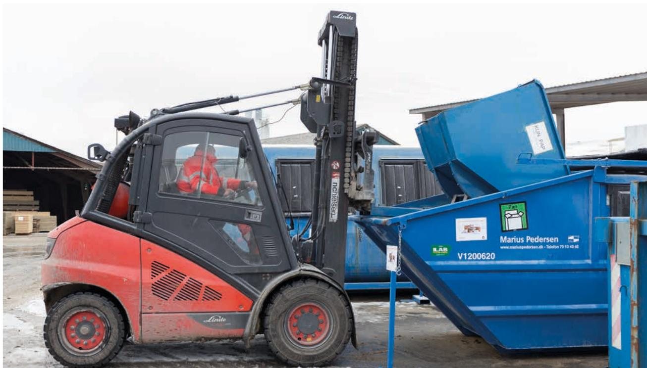
▲ Tipping bins are emptied using a forklift truck, so there is minimal manual handling.
